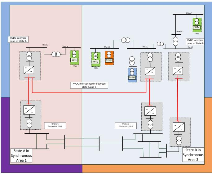
Next to the topology of case 2b, the connection of the two HVDC interface points (isolated AC systems) belonging to different states could be substituted by a common DC connection between the two HVDC stations, as shown in case 2b-2.
