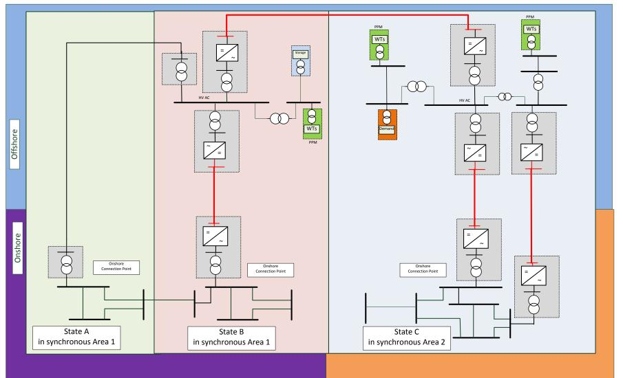
Case 2b: DC coupled HVDC interface points belonging to different synchronous areas
